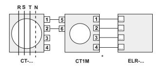
**CT1M:** It's a multiplier for the current setting of those ELR's up to 250 A. It's placed between the ELR and the measuring T/T (It isn't a wire passing through transformer)
