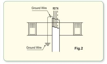
**Nota**: If there is an earthing circuit, it should be placed outside of the T/T (fig1).
